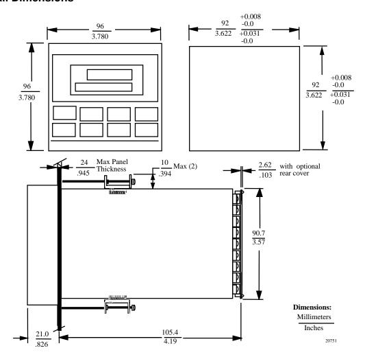
Figure 2-3 Mounting Dimensions (not to scale)
