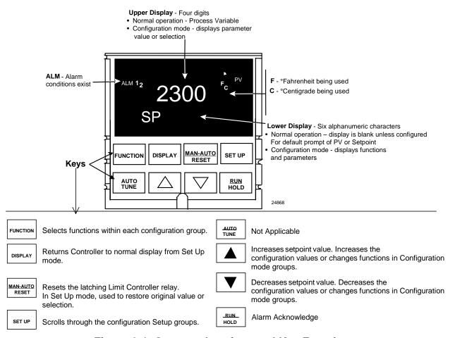
Figure 3-1 Operator Interface and Key Functions
