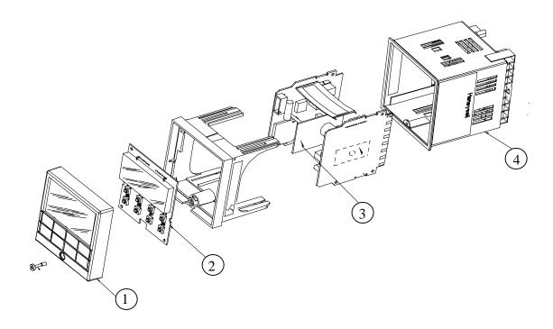
Figure 8-1 UDC2300 Exploded View
