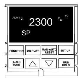
Figure 1-1 UDC2300 Operator Interface
