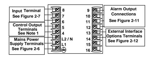
NOTE1: Electromechanical Relay Output – See Figure 2-8 Solid State Relay Output – See Figure 2-9 Open Collector Output – See Figure 2-10
