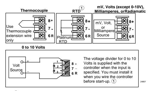
1)These inputs are wired differently than the UDC2000
