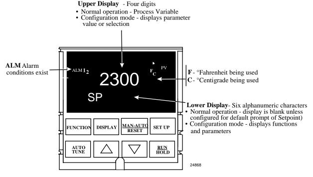
Figure 5-1 Operator Interface
