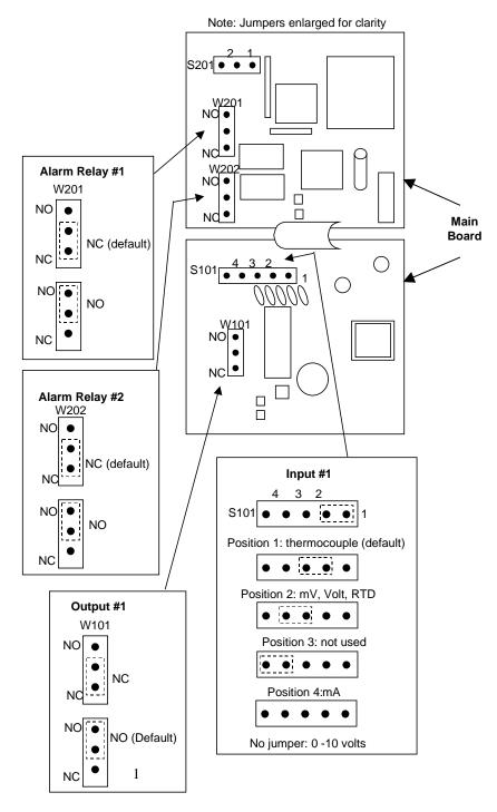
Figure 2-2 Jumper Placements
