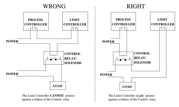
Figure 2-13 Limit Controller Application Diagram
