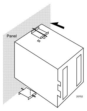
Figure 2-4 Mounting Method
