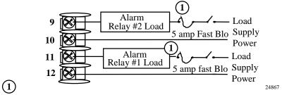
Control relay is configured N.O. as shipped. Alarm relays 1 and 2 are configured N.C. as shipped. N.O. or N.C. configurations are selectable by jumpers on main printed wiring boards. See "Preliminary Checks" in this section of the Product Manual for details.
